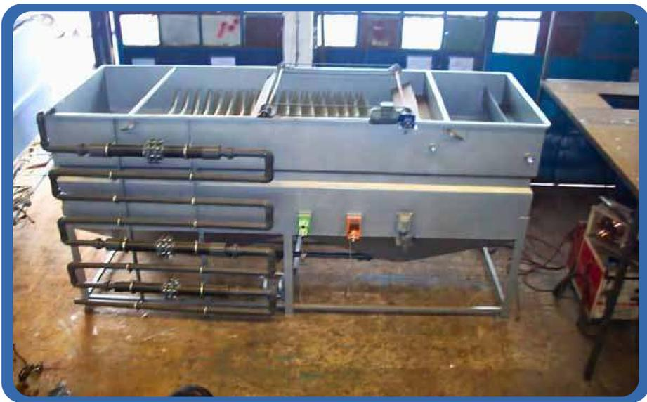
**DGF/DNF – Dissolved Gas flotation unit using nitrogen-gas or biogas in the aeration system**
