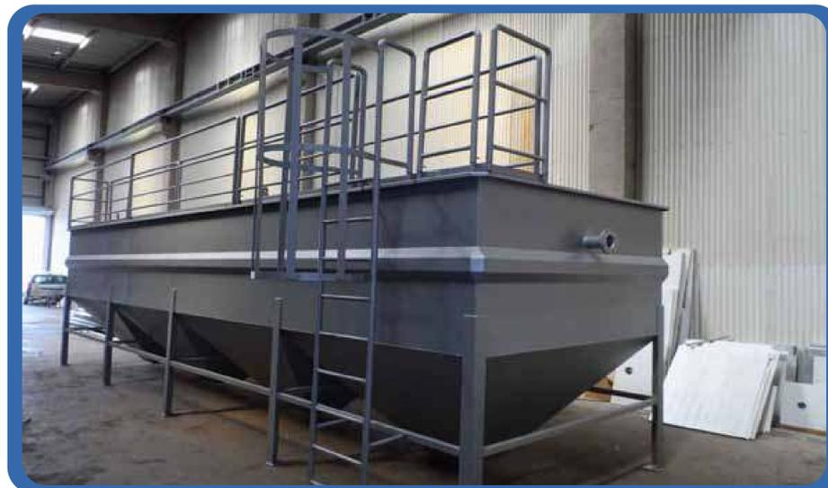
**AECO-FAT – DAF is the first step to recover fat from sludge to be used as biofuel**
